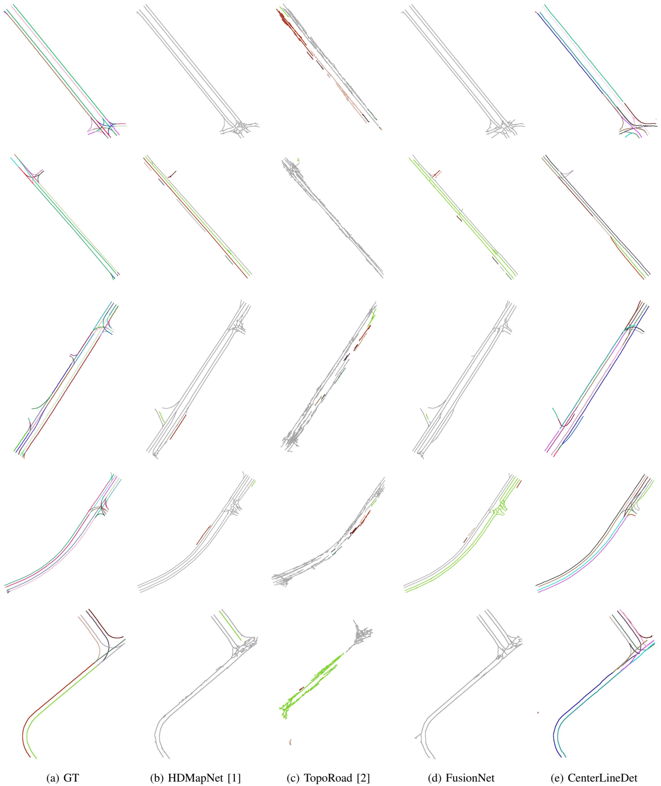
Fig. 10: Qualitative visualizations. Different colors represent different road centerline instances. CenterLineDet is the only approach that can detect and distinguish multiple instances. All baselines mess up different instances, which leads to incorrect topology, especially in the intersection area. For better visualization, graphs are widened but they are actually of one-pixel width. Zoom in for details, especially intersection areas.
