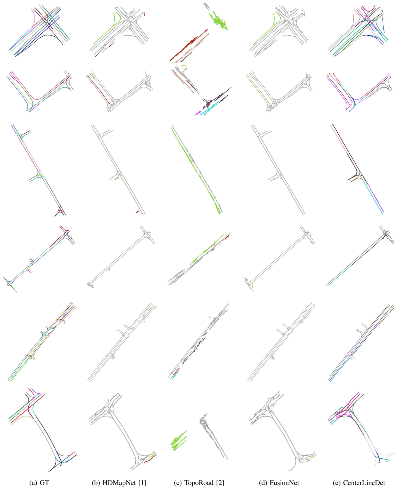
Fig. 9: Qualitative visualizations. Different colors represent different road centerline instances. CenterLineDet is the only approach that can detect and distinguish multiple instances. All baselines mess up different instances, which leads to incorrect topology, especially in the intersection area. For better visualization, graphs are widened but they are actually of one-pixel width. Zoom in for details, especially intersection areas.
