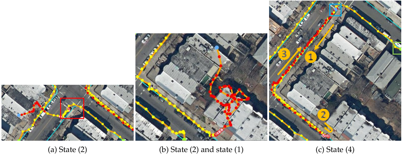
Figure 4: Visualization of the generated graph once uncommon states is not properly handled. For all images, cyan lines are ground-truth curbs. Blue points denote the end vertices and green points denote initial vertices. Orange line segments are edges of the trajectories. Yellow points are normally added vertices, and red points represent vertices that stop action should have been triggered. Red points with pink fill mean that a local infinite loop is detected ( A may or may not escape from the loop).
